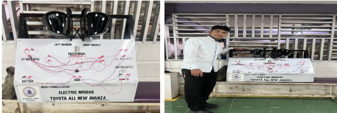
Figure 10. Final Outcome of the Electric Power Mirror Simulator Construction
