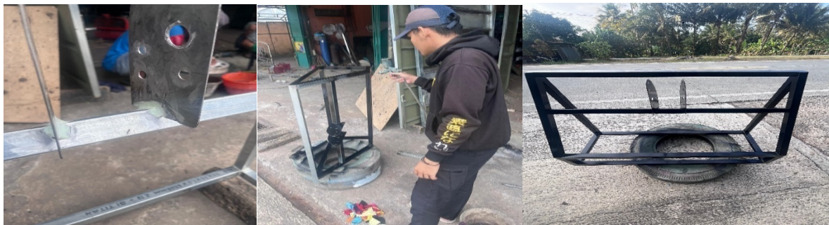
Figure 6. Painting Process of the Simulator Frame
