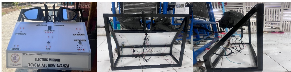
Figure 9. Front, Side, and Rear Views of the Completed Power Mirror Simulator
