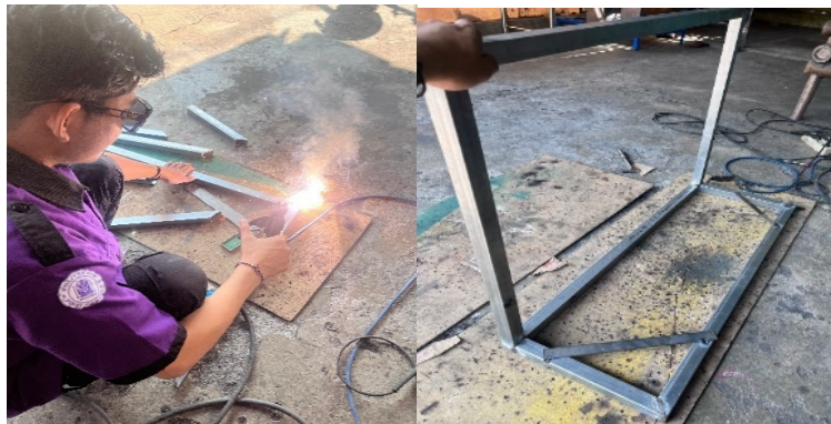
Figure 4. Welding Process of the Simulator Frame
