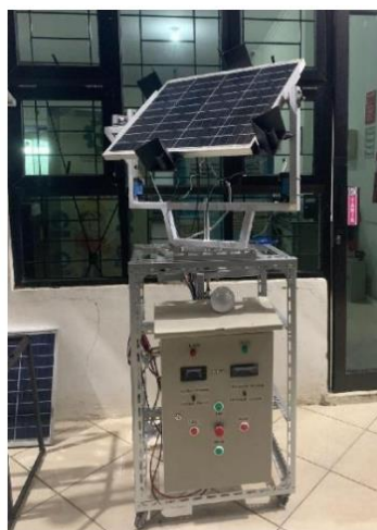
Figure 3. Completed Dual-Axis Solar Tracker Prototype After Assembly
