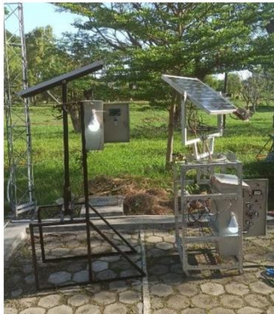
Figure 4. Experimental Setup for Data Collection Comparing Static and Dual-Axis Tracking PV Panels
