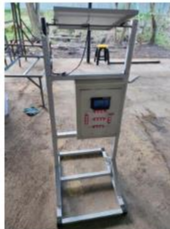
Figure 3. Mechanical Design of the Automated Solar Tracking System
